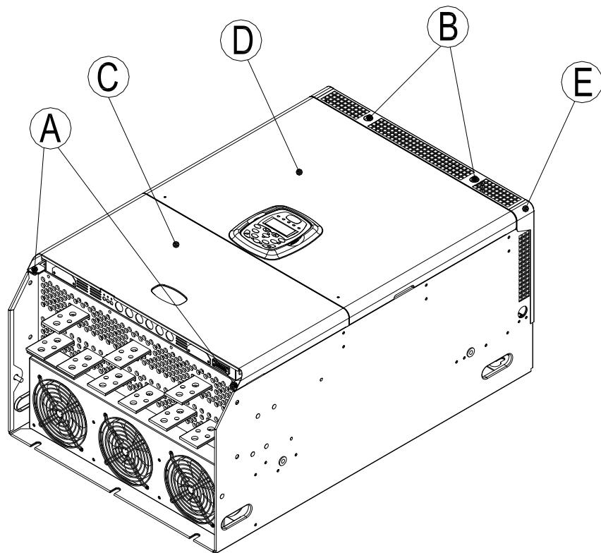
3. Loosen the hex head screws (**F**) and remove the main cover (**D**) from the inverter.
