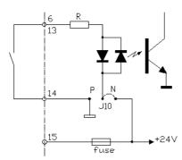
NPN command (active to zero Volt) through voltage – free contact.
