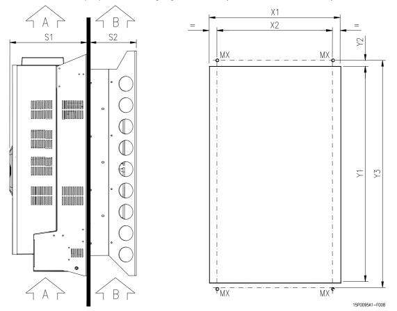
Figure 7: Through-panel assembly and piercing templates for SINUS K S15 and S20.
