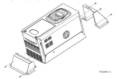
Figure 5: Mounting the accessories for SINUS K S12 through-panel assembly.
