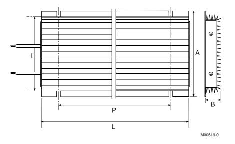
Figure 15: Overall dimensions and mechanical features for braking resistors from 1100W to 2200W.
