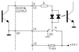
NPN command (active to zero Volt) sent from a different device (PLC, digital output board, etc.)
