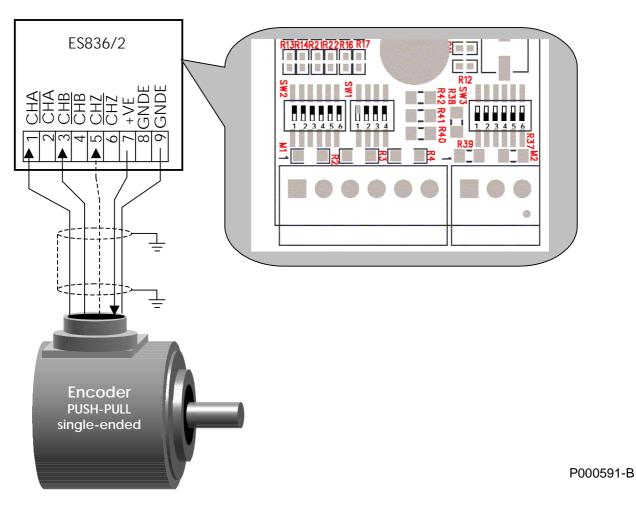
Figure 28: PUSH-PULL encoder with single-ended outputs.
