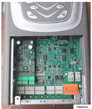
Figure 25: Encoder board fastened to its slot.
