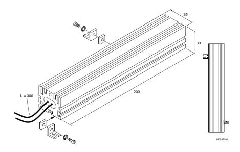
Figure 13: Overall dimensions, 56-100 $\Omega$ /350W resistor.
