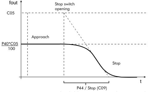
Figure 46: Frequency produced while stopping in Normal operating mode.
