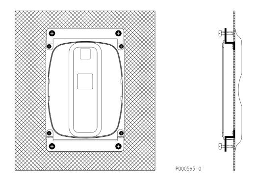
5 – Remove the display/keypad from the inverter (see figure below). A short wire with 8-pole telephone connectors is used to connect the display/keypad to the inverter. Press the cable tab to disconnect it.
