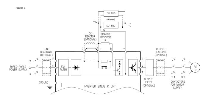
Figure 33: Wiring diagram for EU850 unit.
