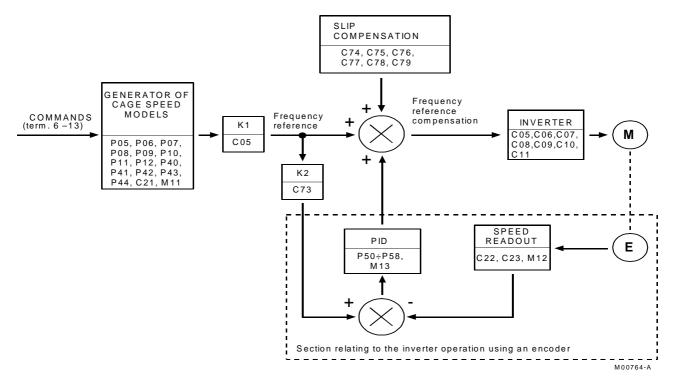
Figure 34: Block diagram of the speed regulator.
