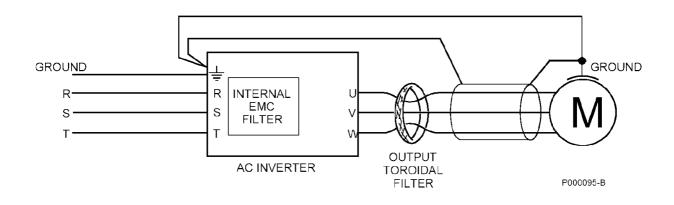
Figure 54: Wiring the toroid filter for the inverters of the SINUS K series.
