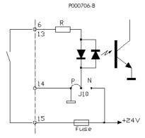
PNP contact (active to +24V) through voltage -free contact.
