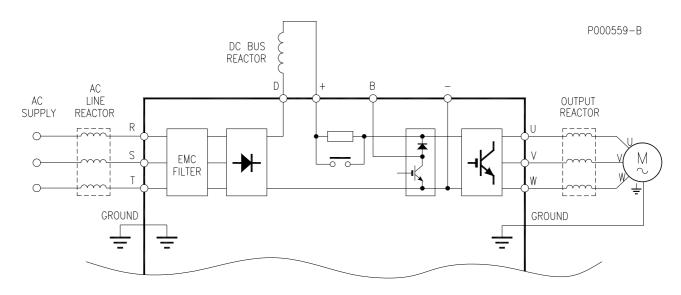
Figure 19: Wiring diagram for optional inductance.
