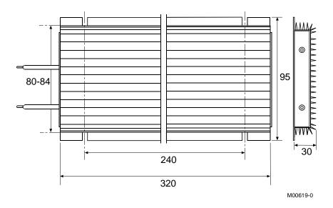
Overall Dimensions, Resistor 1100W - IP55
