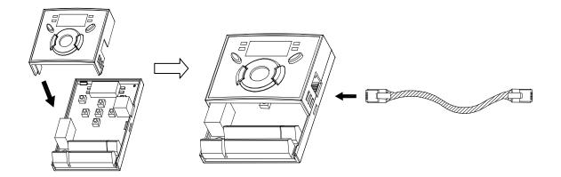
3) Connect the other side of the remote cable to the remote keypad as shown below.
