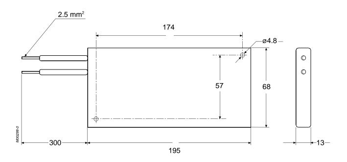
Overall Dimensions, Resistor 550W - IP55
