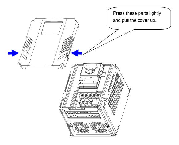
To change the inverter fan: Press the both sides of bottom cover lightly and pull out .
