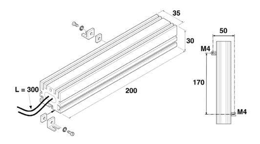
Overall Dimensions, Resistor 350W - IP55
