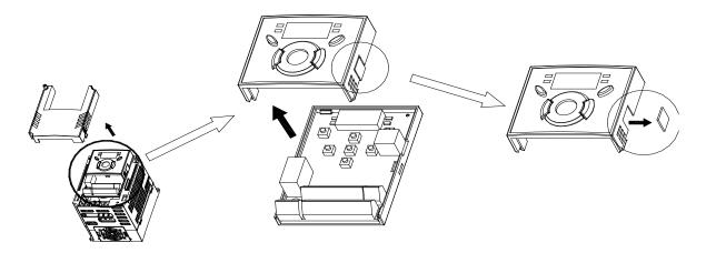
2) Attach the top cover of the I/O board kit and connect the remote cable as shown below.
