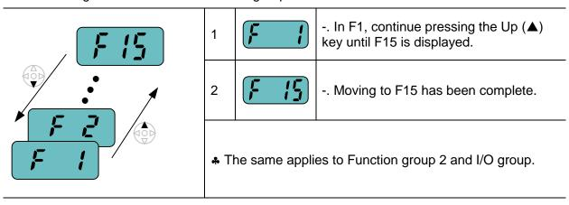
♣ Note: Some codes will be skipped in the middle of increment (▲)/decrement (▼) for code change. That is because it is programmed that some codes are intentionally left blank for future use or the codes user does not use are invisible.
