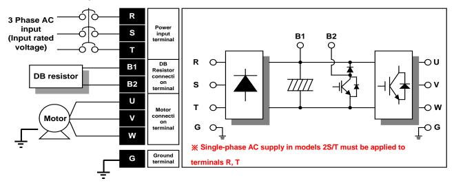
Power terminal wiring (11.0 ~ 22.0kW)
