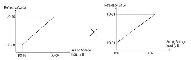
$$FBK \ display = \left( \left( \frac{I10 - I8}{I9 - I7} \right) \times \left( Input \ Voltage - I7 \right) + I8 \right) \times \frac{(I90 - I89)}{MaxFreq} + I89 \quad when \ feedback \ is \ from \ V1 = I8 + I89 = I89$$
